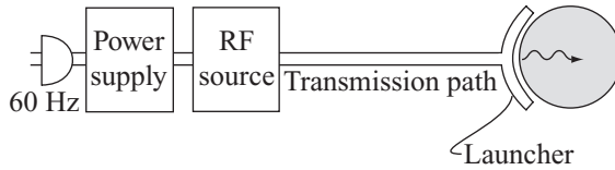
Figure 15.7 Schematic diagram of an RF heating or current-drive system.
