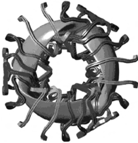
Figure 13.48 Schematic diagram of the NCSX in the USA (courtesy of A. R. DeMeo).
