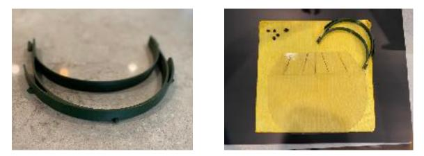
The image shows the frame and it can be seen that a space exists between the forehead area and the outer rim that retains the shield. This allows loops to be worn but allows aerosols to enter from above the shield. The pattern traced on the vinyl was created using a cardboard pattern and the traced onto the vinyl. It is important to do work on a microfiber towel to avoid inadvertent scratches to the vinyl material.
