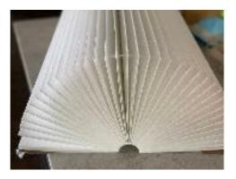
Figures 9-10 filter material, no cardboard or wire mesh only fibrous cellulose Merv 11 filter material to deal with.
