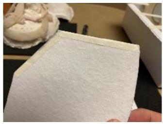
Figures 11-12 Pattern taken from KN95 and transferred to Merv 11 filter paper for cutting
