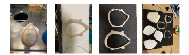
Figures 5-8 Beginning mask frame, finished frame, comparison of Bellus and models and frames with cut out of Merv 11 fibrous cellulose filter material.
