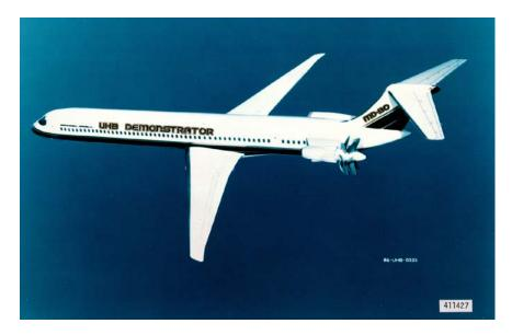
Figure 4-8. The McDonnell Douglas MD-80 UHB Demonstrator is shown with the 578-DX engine. (NASA)
