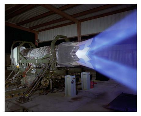
Figure 6-2. This image shows the Pratt & Whitney F119 Engine for the F-22. (Pratt & Whitney)
