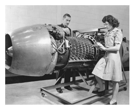
**Figure 1-10.** Captured German jet technology, especially the Junkers Jumo 004B axial-flow turbojet, was of considerable interest to NACA researchers at the Aircraft Engine Research Laboratory in the immediate post–World War II period. (NASA)
