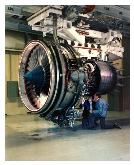
GE's  $E^{\rm 3}$  demonstrator of 1983 reflected advances in fuel efficiency and noise and emissions reductions that benefited from NASA support and research in turbofan development. (NASA)
