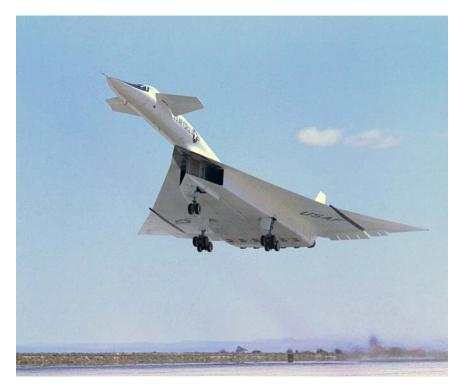
**Figure 2-3.** The XB-70 was the world's largest experimental aircraft when the Air Force and NASA partnered to use the canceled bomber as a flying laboratory to generate data for future supersonic aircraft. The controllable internal geometry of the inlets maintained efficient airflow to the six YJ93 turbojets. (NASA)
