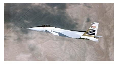
Dryden researchers used a NASA F-15 to test the Digital Electronic Engine Control (DEEC) system from 1981 to 1983. (NASA)
