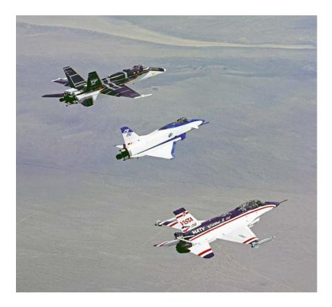
Figure 5-10. Shown are the F/A-18 HARV, the X-31, and the F-16 MATV, all thrust-vectored research aircraft. (NASA)
