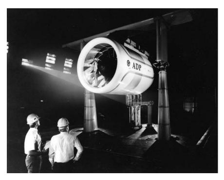
**Figure 6-4.** The Pratt & Whitney and NASA team prepare the Advanced Ducted Propulsor (ADP) for a flow visualization test in the National Full-Scale Aerodynamics Complex (NFAC) 40- by 80-foot Wind Tunnel at the Ames Research Center. (NASA)
