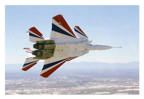
**Figure 5-9.** The Pratt & Whitney pitch-yaw balance beam nozzle system enabled vectoring horizontally (yaw) and vertically (pitch). The ACTIVE program achieved the first supersonic yaw-vectoring flight on April 24, 1996. (NASA)
