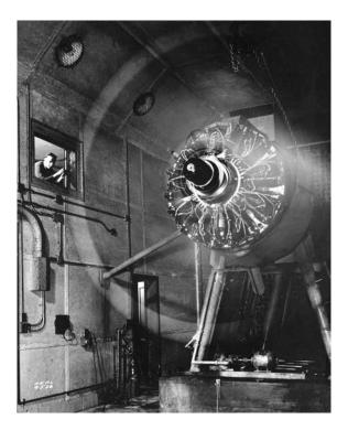
**Figure 1-5.** The Aircraft Engine Research Laboratory in Cleveland, OH, supported the United States aviation production program during World War II. Much of the development work involved straightforward evaluation of propeller-and-engine combinations on torque stands to determine their overall power. (NASA)
