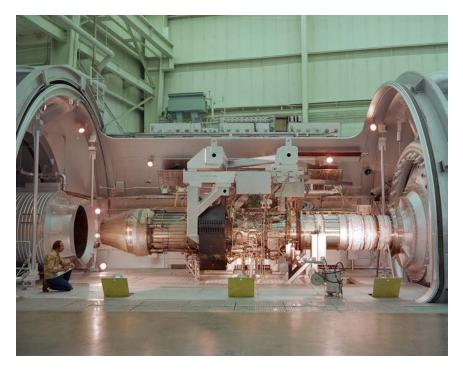
Figure 2-9. This image shows a Pratt & Whitney F100 engine installed in the much larger PSL No. 4 in 1981. (NASA)
