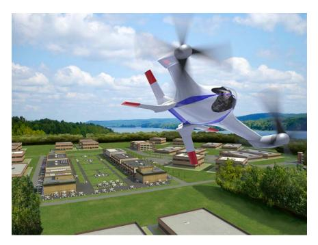
Figure 7-4. The Puffin is designed to be a personal aircraft. (NASA/Mark Moore)
