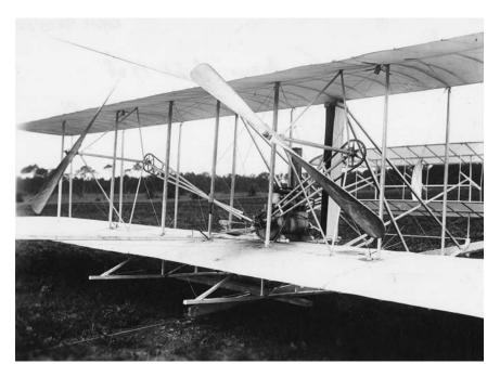
**Figure 1-1.** While they emphasized their Flyer's control system as their unique contribution to the development of flight, the Wrights' propellers were equally revolutionary. (National Air and Space Museum, Smithsonian Institution, NASM 9A05000)
