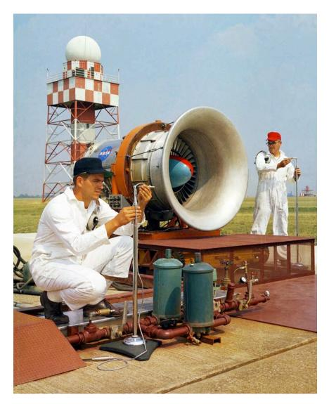
NASA technicians prepare for a jet engine noise test on the airfield at Lewis Research Center in 1967. (NASA)  $% \left( \left( A_{1}^{2}\right) \right) =0$
