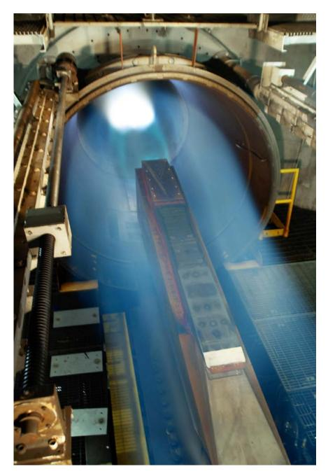
Figure 6-6. The Pratt & Whitney Rocketdyne SJX61-2 scramjet undergoes ground testing simulating Mach 5 flight conditions in the Langley 8-Foot High Temperature Tunnel. (NASA)
