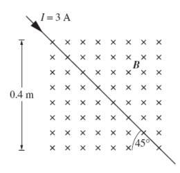
What is the magnitude of the magnetic force on the conductor?
