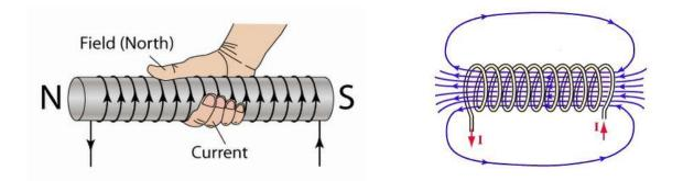
Note that a current-carrying solenoid produces a dipole field similar to that of a bar magnet. The field is uniform within the coil.
