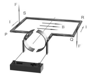
The diagram above shows a simplified D.C. motor. Note that in the position shown, the plane of the coil is *parallel* to the magnetic field.
