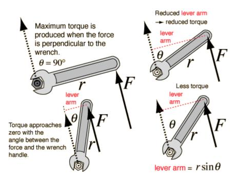
Torque on wrench = Force x lever arm
