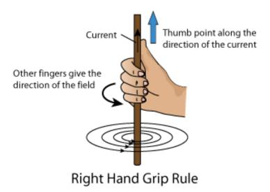
This rule may also be used 'in reverse' to determine the direction of the magnetic field within a current-carrying coil (solenoid). Here, the fingers of the right hand curve in the direction of the current in the coil windings, and the thumb points in the direction of the magnetic field.
