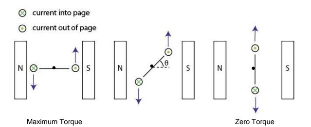
The magnitude of the torque acting on a current-carrying coil in a magnetic field is given by:
