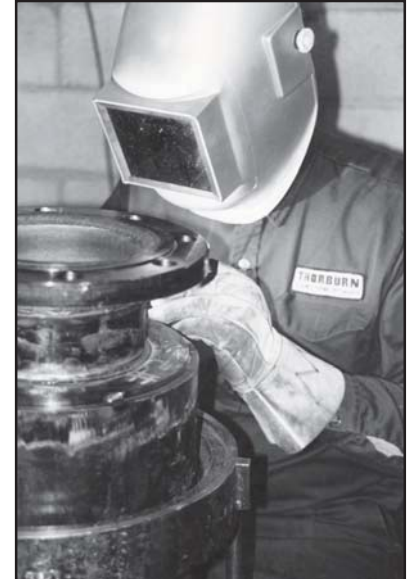
Thorburn's state-of-the-art TIG welding technology for externally pressurized expansion joint assembly
