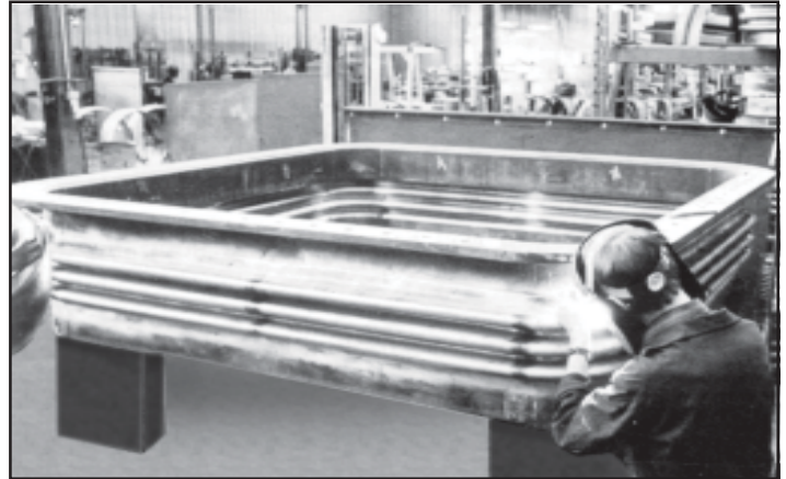
Welding of a typical Thorburn round radius corner rectangular expansion joint Series FRU
