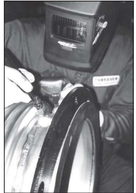
Thorburn's skilled welder certified to ASME Section IX using modern TIG welding for bellows flange attachment
