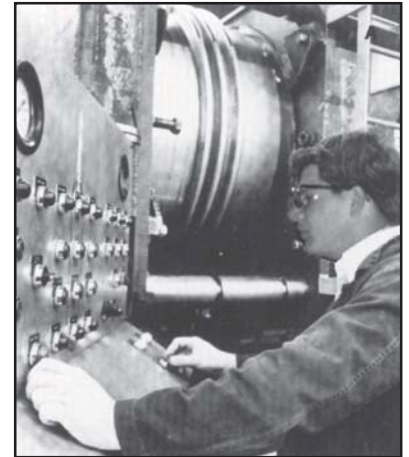
Hydro forming bellows from a metallic tube for nuclear ASME Section III service
