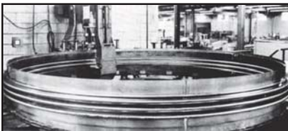
Large diameter roll forming of bellows
