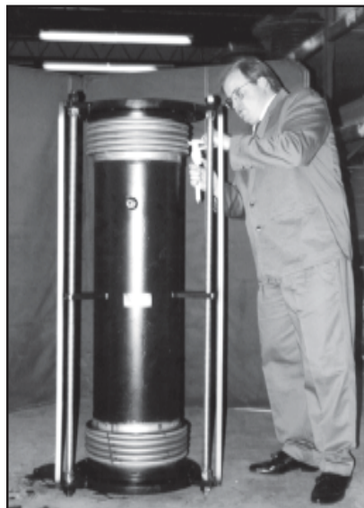
Thorburn flexible piping specialist verifying bellows' integrity
