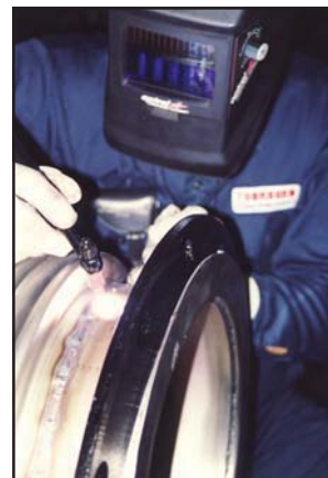
Thorburn's procedures and welders certified to ASME Sections III, VIII, IX using modern TIG welding technology
