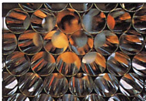
Bellows tubes prior to convolution forming
