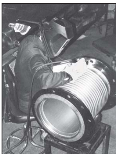
Thorburn welders and welding procedures to ASME Section III, VIII and IX
