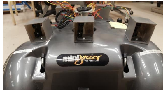
FIGURE 13: IR Sensor mounted on wheelchair [4]
