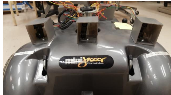
FIGURE 2: IR-Sensor Mounted on wheelchair [4]
