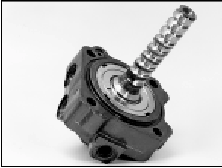
Inspect input shaft, valve/worm assembly sealing areas
