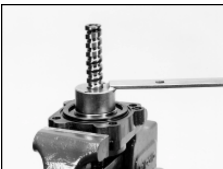
Remove bearing adjuster
