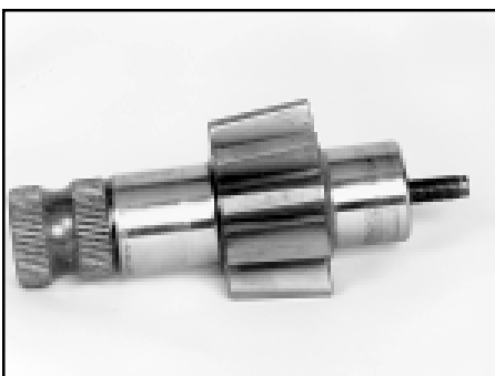
Inspect sector shaft assembly
