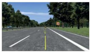
**Fig. 5:** Visualization of intentions (potential trajectories and speed limits) of a highly automated vehicle in a contact-analogue head up display (Damböck et al. 2012b).
