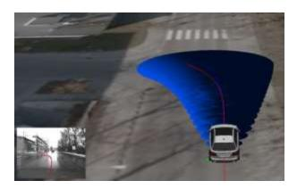
**Fig. 7** Ego-vehicle trajectory prediction using the Trajectory history and present sensor signals like steering angle and yaw rate.
