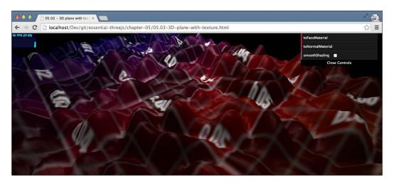
This mapping is based on the UV information we specified. So, if you create a custom geometry, remember to also think about how a texture should be applied to it. Now we can very easily create very interesting-looking terrains. For instance, the following figure was created with a simple wood-like texture (05.03-3D-plane-with-texture.html):
