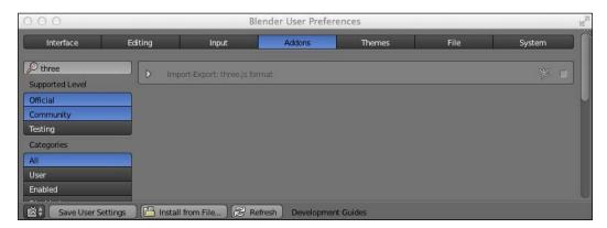
Here, you can see that the Three.js plugin is found, but as it is gray in color, it isn't enabled yet. You can now enable the plugin by checking the checkbox to the far right, as shown in the following screenshot:
