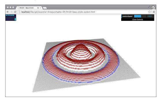
In this screenshot, we've got a particle system that shows the volume of the low, mid, and high ranges. In the middle of the screenshot, you can see the volume of the low range. The middle ring shows the volume of the mid range, and the outer ring shows the high notes.
