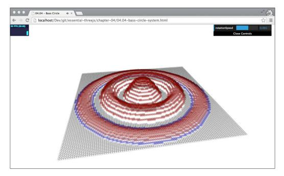
The visualization you can see in the previous screenshot shows the low, mid, and high tones of the audio that is being played in the form of concentric circles. The low tones are shown in the center of the visualization, the second circle shows the mid tones, and the outermost circle shows the amplitude of the high tones. To create this visualization, we have to perform the following steps:
