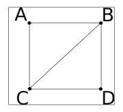
As you can see in the figure, we are going to create squares by combining two faces. So we need to create a face using the **A**, **B**, and **C** vertices, and another face using the **B**, **C**, and **D** faces. We do this in the following code fragment:
