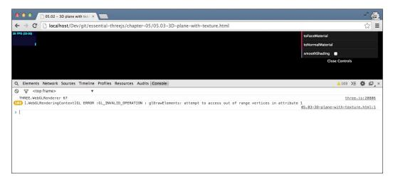
The reason, which isn't actually clear from this error message, is that we're missing one more piece of configuration in the geometry we've created: the UV map.
