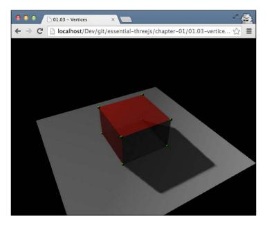
Here, each vertex is shown as a small green sphere. So, when we create a THREE. CubeGeometry object, we actually create eight vertices.
