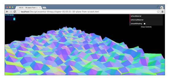
In this example, you can also enable smoothShading. With smoothShading, you don't see the individual faces, but Three.js combines them to create a smooth geometry. You can easily enable this by setting the shading property of the material to THREE.SmoothShading. The result looks like the following screenshot:
