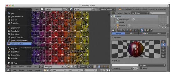
Each black dot you see in this square represents a vertex of the model, and you can see how each face is mapped to the texture. Now that we've set up UV mapping, we can export the model to Three.js and render it.
