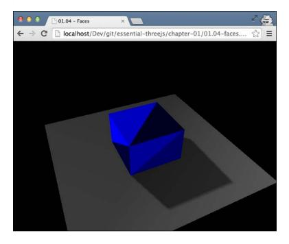
Here, you can see that each side of the cube is divided into two faces, and the corners of each face are defined by a vertex.
