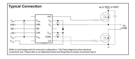
Figure 7: MOSFET driver circuit
