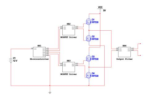
Figure 3: Basic Component Diagram
