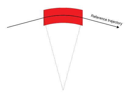
Consider the magnetic field close to the entrance pole face of a dipole. We consider an arbitrary rotation of the pole face through angle  $\psi$  from the normal to the reference trajectory.
