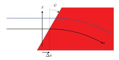
A particle travelling parallel to the reference trajectory but with some positive horizontal offset does not see the main bending field of the dipole until some time later than a particle travelling exactly along the reference trajectory. The result is that the first particle is no longer travelling parallel to the reference trajectory: there is an effective deflection proportional to the horizontal offset of the particle.
