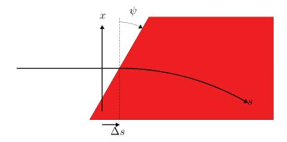
The effect of the fringe field (including the pole face rotation) is contained within the region  $0 < s < \Delta s$ , and is represented by the magnetic field:
