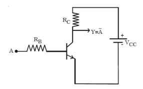
32. Give the Boolean equation for the given logic diagram.
