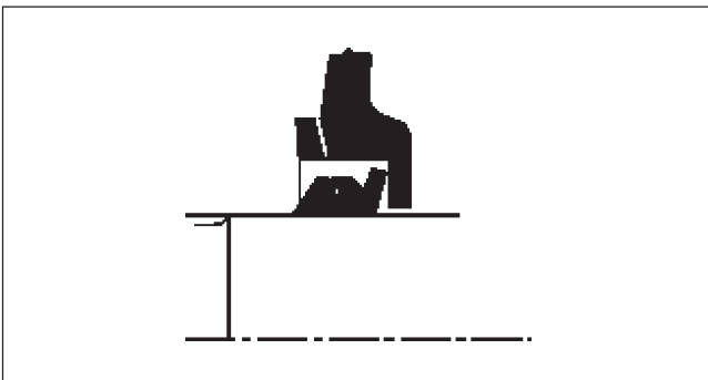
Dismantling the V-ring and adjacent protecting ring
