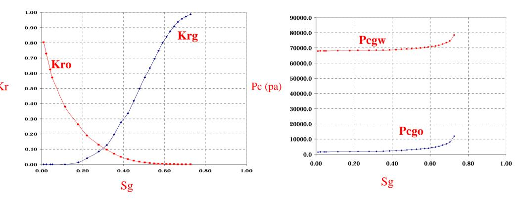
Results for the Berea sandstone network for secondary gas injection
