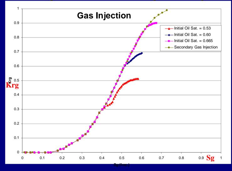
Effect of initial oil saturation on gas relative permeability
