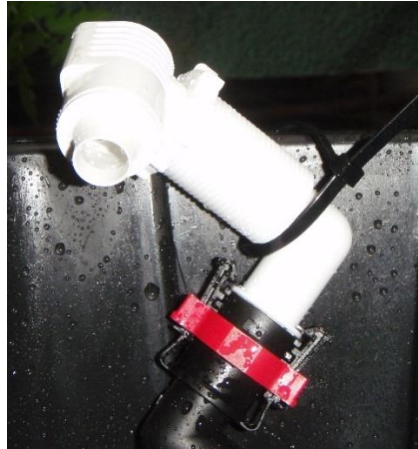
Figure 30- Aeration Nozzle Attached to Reservoir
