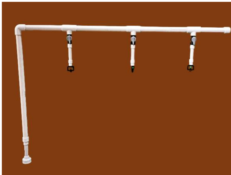
Figure 20-Top Portion of Supply Line without splashguards
