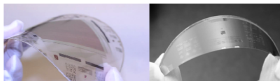
Fig. 2: Flexible electronics on flexible plastic (PEN, left) and stainless steel (right) substrates
