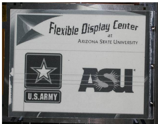
Fig. 1: An active matrix QVGA electrophoretic display fabricated on flexible stainless steel.
