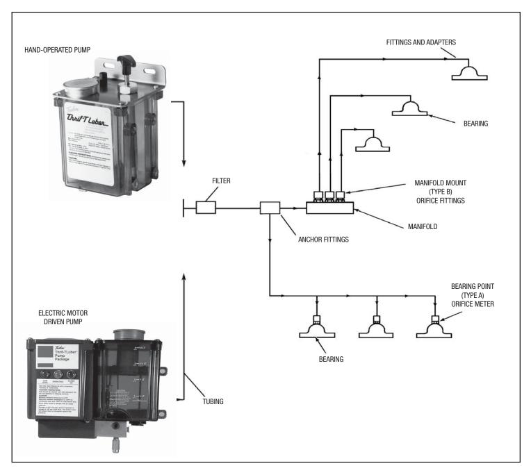
Figure 1: Thrif-T Luber System Diagram
