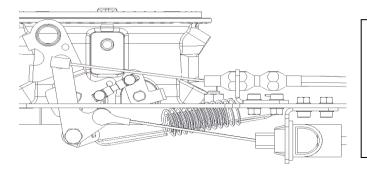
Note: Some cables require the cable length to be set by adjusting the cable end stop. If you are using this style cable, loosen the set screw on the cable end stop and slide it until it is touching the transmission cable clip. Now tighten the set screw and follow the adjustment procedure above.
