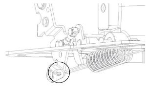
4. Select the throttle cable bracket for your application, then use washers between the bolt heads and nuts and loosely mount the throttle cable bracket to the base plate. Then insert the throttle cable.
