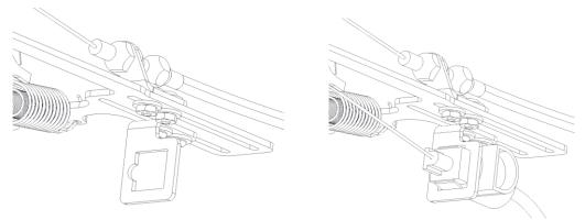
7b. Clip the transmission cable to the stud on the corrector. Adjust the cable using the OEM procedure if possible. Otherwise, adjust the location of the transmission bracket to ensure that the cable is pulled all the way out at full throttle. While the transmission cable is correctly adjusted, tighten the transmission bracket mounting bolts. Be sure to use the supplied washers underneath the bolt heads and nuts. Installation is complete.
