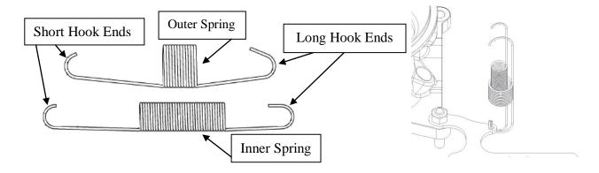
3. Rotate the springs downward to attach the loose ends to the throttle lever spring hole as shown. Long hook ends should be routed underneath the base plate.
