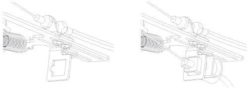
7c. Clip the cable end to the OE transmission cable stud on the throttle lever and adjust the cable using the OEM procedure if possible. Otherwise, adjust the location of the transmission bracket to ensure that the cable is pulled all the way out at full throttle. While the transmission cable is correctly adjusted, tighten the transmission bracket mounting bolts. Be sure to use the supplied washers underneath the bolt heads and nuts. Installation is complete.
