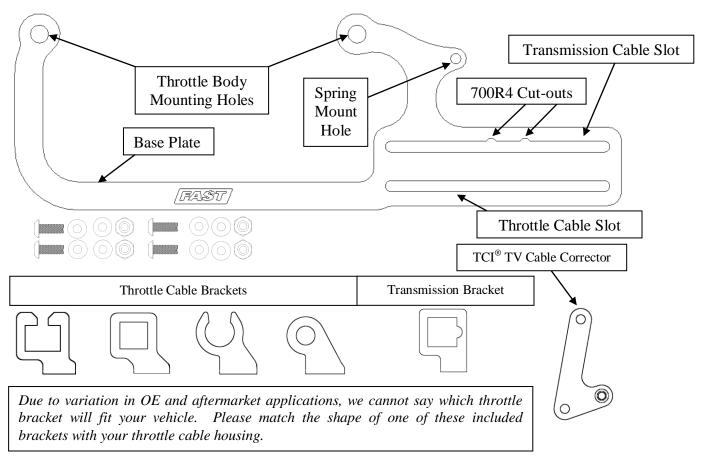
1. Place the base plate over the studs with the logo facing up, then replace and tighten the nuts.
