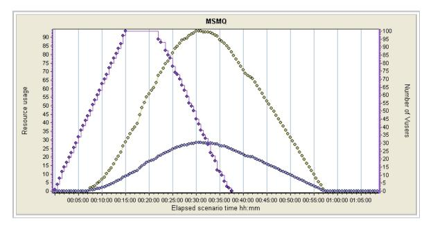
The purple line shows the number of Vusers. The yellow line shows the number of transactions in the MSMQ queue awaiting execution. The gray line shows another processing component of MSMQ. It is interesting to note that queuing occurs at the same level of load in both configurations, i.e., 49 simultaneous Vusers. At this point, the application is saturated.
