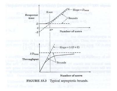
In this diagram,  $N^*$  is the number of users (an expression of load) at which the application begins to go into saturation. It is also sometimes referred to as the point of optimal throughput. D is the service demand, which will be discussed below,  $D_{max}$  is the maximum service demand of all of the devices in the application, again discussed below, and Z is user 'think time' (not important to this discussion).
