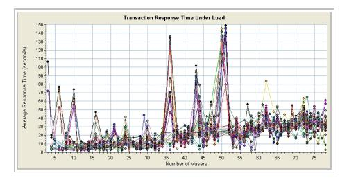
In this particular example, the available memory on the application server was extremely low, reaching a minimum of 2 MB available out of a total of 1 GB. The CPU utilization on the application server was also extremely high. Once again, we can see that the application is starting to go into saturation at about 30 Vusers.
