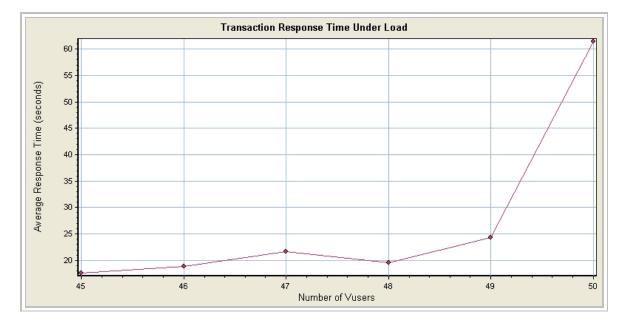
This chart was taken from an actual load test. It is important to always generate this chart in LoadRunner in order to diagnose whether or not the application is saturating. Here, the application goes into saturation at a load equivalent to 49 simultaneous virtual users, where the operations performed be each virtual user are designed to mimic as closely as possible the mix of operations performed by actual users.
