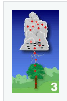
Lightning channel develops
