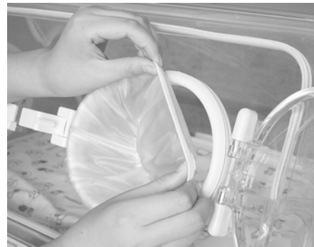
INSTALLATION OF ACCESS DOOR CUFF
