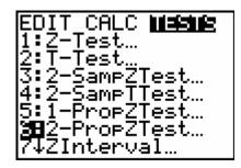
Enter in the data for the 2-PropZTest. Highlight Calculate and press the **ENTER** key. 2-PropZTest ×1:100 n1:500 ×2:68 n2:400 p1:≠p2 <p2 **№20** Calculate Draw
