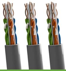
APPLICATIONS: Suitable for enterprise applications designed to deliver robust standards based performance ensuring optimum bandwidth for today's high speed network applications. The cable is designed to support horizontal networking applications over distances up to 100 meters, 10GBASE-T Ethernet. Fully compliant to Category 6A requirements, including alien crosstalk (AXT).
