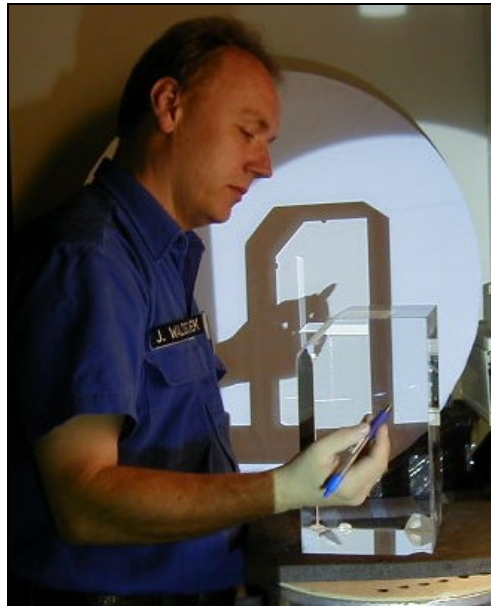
Figure 4: Striae testing using the shadowgraph method.
