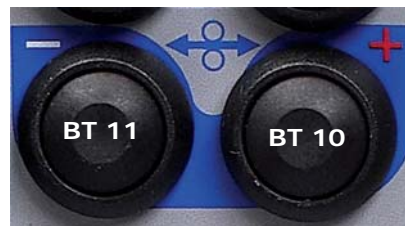
Fig. 5.2 - Controls used for positioning the filler wire
