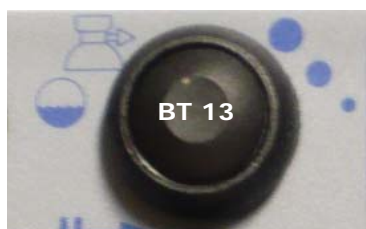
Fig. 5.4 - Push button for testing gas - testing coolant - and restarting the coolant pump
