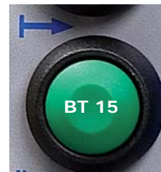
Fig. 5.7 - Pushbutton to control cycle start
