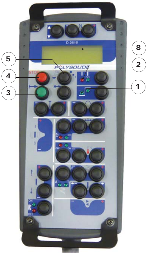
Fig. 6.12 - View of P6 HW remote control front panel
