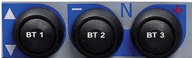
Fig. 5.5 - Controls used for selecting the WP/program
