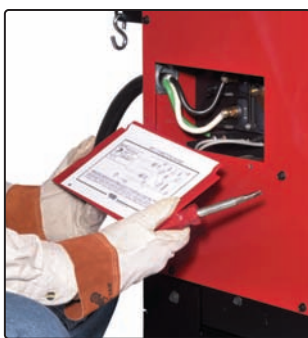
Easily accessible input voltage reconnect panel.
