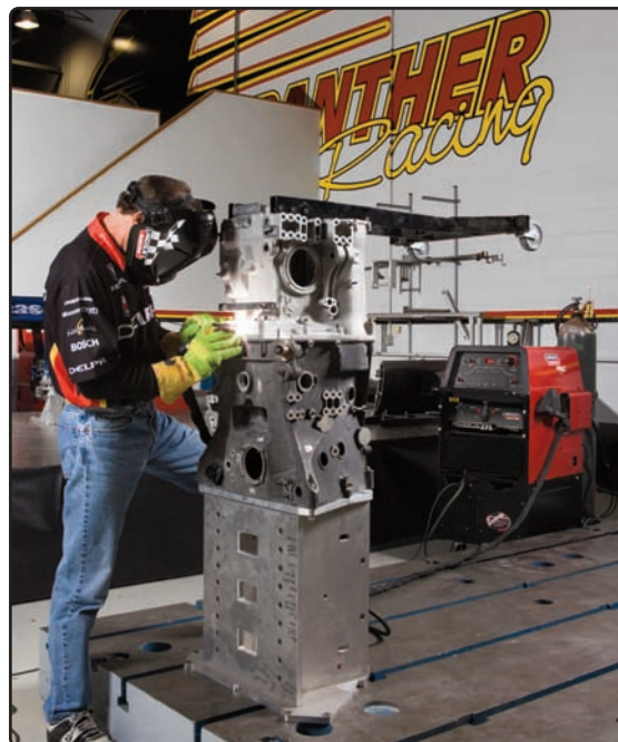
AC Auto Balance® is especially useful on critical aluminum applications.
