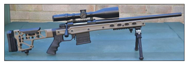
To complete the build, I fitted an Atlas bipod, which in my opinion are one of the best bipod's on the market, scope rings where German 30mm Rechnagel which although relatively expensive are of excellent quality and the scope was a German Tactical KAPS 2.5-10x56.
