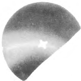
Straight directional break due to defective material. Full credit is granted at original purchase price.
