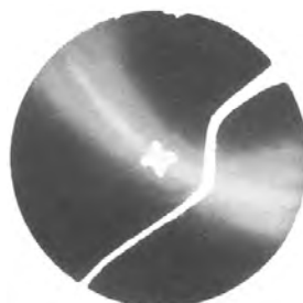
Disk fracture resulting from contact with rocks, stumps, or other solid objects. Credit is not offered.
