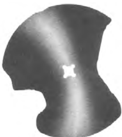
Disk fracture resulting from contact with rocks, stumps, or other solid objects. Credit is not offered.
