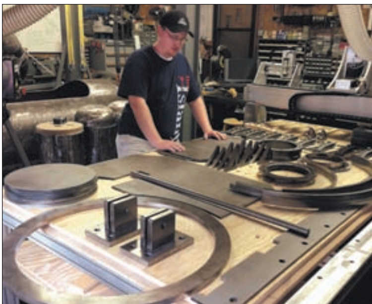
Piecing together the puzzle – Widman surveys a table full of laser cut steel components for the sub.
