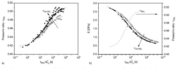
Figure 12. a) Poisson's ratio,  $v_{\text{REL}}$ , and b) relaxation modulus, *E*, master curves as a function of reduced relaxation time at a reference temperature  $T_0 = 30^{\circ}$ C for two different axial deformations  $\varepsilon_{\text{AX,REL}}$ : 0.005 ( $\circ$ ) and 0.01 ( $\bullet$ )
