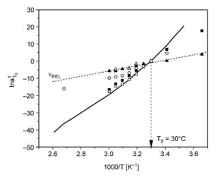
Figure 13. Shift factors employed for the construction of the following master curves: a) storage modulus vs. frequency, b) Poisson's ratio v<sub>CDR</sub> vs. strain rate, c) Poisson's ratio v<sub>REL</sub> vs. t<sub>REL</sub> (ε<sub>AX,REL</sub> = 0.005 (▲) and 0.01 (■)) and E vs. t<sub>REL</sub> (ε<sub>AX,REL</sub> = 0.005 (△) and 0.01 (□))
