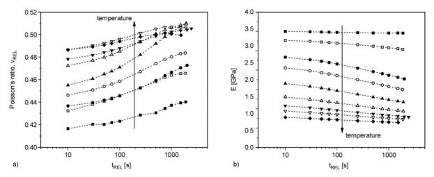
**Figure 11.** a) Isothermal Poisson's ratio,  $v_{REL}$ , and b) relaxation modulus, *E*, isothermal curves as a function of relaxation time,  $t_{REL}$ , at various temperatures: 0°C ( $\blacksquare$ ); 20°C ( $\square$ ); 30°C ( $\bullet$ ); 35°C ( $\circ$ ); 40°C ( $\blacktriangle$ ); 45°C ( $\Delta$ ); 50°C ( $\triangledown$ ); 55°C ( $\nabla$ ); 60°C ( $\blacklozenge$ ); data obtained for an axial deformation  $\varepsilon_{AX,REL} = 0.01$
