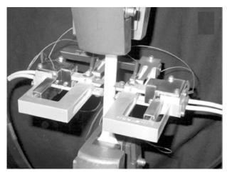
Figure 2. Experimental set-up employed for the Poisson's ratio measurement, in adoption of a clip-on biaxial extensometer (Instron mod. 2620) mounted on a PBT dumb-bell specimen
