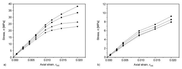
Figure 5. PBT isochronous stress *vs*. strain curves at a) 30°C and b) 70°C for various instants: 10 s (■); 100 s (●); 1000 s (▲); 1 h (▼)
