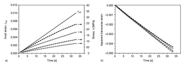
Figure 6. Time evolution of a) axial strain, ε<sub>AX</sub>, and stress, σ, and b) apparent transverse strain in CDR experiments for an axial strain rate of 0.003 s<sup>-1</sup> at various temperatures: 20°C (**□**); 30°C (**□**); 50°C (**△**); 60°C (**△**)
