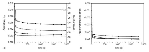
Figure 7. Time evolution of a) axial strain,  $\varepsilon_{AX}$ , and stress,  $\sigma$ , and b) apparent transverse strain in REL experiments carried out at  $\varepsilon_{AX,REL} = 0.01$  at various temperatures: 20°C (**a**); 30 °C(**b**); 50°C (**A**); 60°C(**b**)
