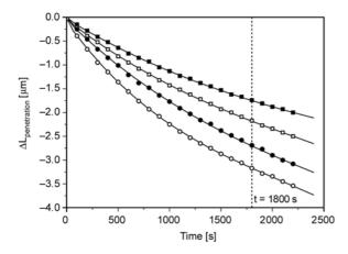
Figure 8. Transverse displacement due to the extensioneter lateral penetration measured on an undeformed specimen as a function of time at various temperatures: 30°C (■); 40°C (□); 50°C (●); 60°C (○)
