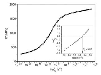
Figure 4. E' master curve as a function of reduced frequency at a reference temperature,  $T_0 = 30^{\circ}$ C; insert: shift factors evaluated by best superposition of isothermal E' vs. frequency curves
