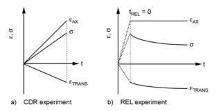
**Figure 1.** Schematic representation of input (axial deformation,  $\varepsilon_{AX}$ ) and output (stress,  $\sigma$ ; transverse deformation,  $\varepsilon_{TRANS}$ ) variables in a) constant deformation rate (CDR) experiments and b) constant deformation (REL) experiments
