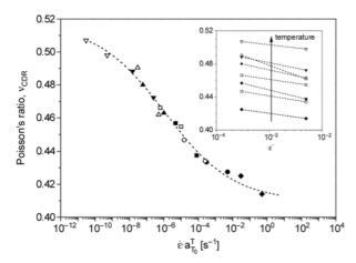
Figure 10. Viscoelastic Poisson's ratio, v<sub>CDR</sub>, master curve as function of reduced strain rate at a reference temperature T<sub>0</sub> = 30°C after shifting of the isothermal curves at temperatures: 20°C (♦); 30°C (●); 35°C (○); 40°C (■); 45°C (□); 50°C (▲); 55°C (Δ); 60°C (▼); 100°C (∇); insert: isothermal curves before shifting
