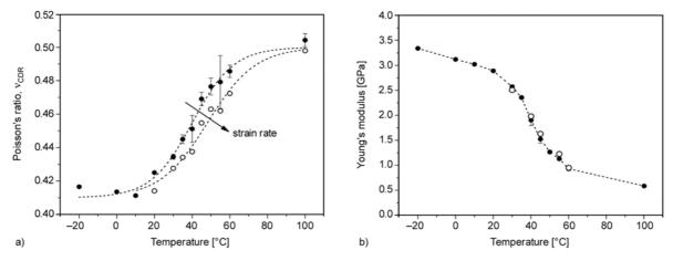
Figure 9. a) Viscoelastic Poisson's ratio,  $v_{CDR}$ , and b) Young modulus for semicrystalline PBT evaluated at different deformation temperatures along a deformation ramp at strain rate of 0.003 s<sup>-1</sup> (•) and of 0.05 s<sup>-1</sup> ( $\circ$ )
