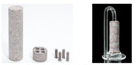
FIGURE 1: Drill core and specimens (left). Cylindrical specimens between push rod and sample table in the analyzer TMA 402 F3 Hyperion Netzsch (right).
