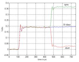
**Fig. 5** Calibration Standards for S<sub>11</sub> TDR measurements. Short Circuit (red), Open Circuit (green), and 50 Ω Termination (blue)
