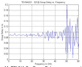
Fig. 11 TDVNA S<sub>21</sub> Group Delay measurement of 6 dB, K attenuator
