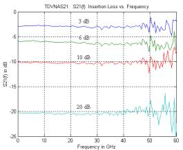
**Fig. 10** TDVNA S<sub>21</sub> Insertion Loss measurements of precision PSPL model 5510K, 3 dB, 6 dB, 10 dB, and 20 dB, 2.95mm coax attenuators
