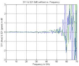
Fig. 9 TDVNA system 0 dB self-test of repeatability and max. frequency. Test conditions were: N=4096,  $T_w = 2 \text{ ns}$ , 256 averages. S<sub>21</sub> (green), S<sub>11</sub> (blue)
