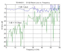
Fig. 12 TDVNA  $S_{11}$  Return Loss measurements of precision 3 dB K attenuator terminated in 50  $\Omega$  (green) and a short circuit (blue)
