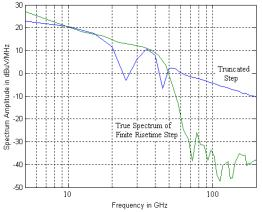
**Fig. 2** Spectrums of Step-Like Waveforms. The example shown is a PSPL model 4022 TDR pulser measured by an HP 50 GHz oscilloscope.
