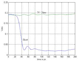
**Fig. 6** Optimum positioning of TDVNA TDR, S<sub>11,</sub> waveforms on oscilloscope screen
