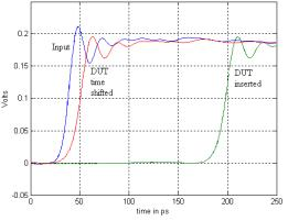
Fig. 7 Optimum positioning of TDVNA TDT,  $S_{21}$ , waveforms on oscilloscope screen
