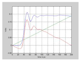
**Fig. 3** The Nicolson method [8] of subtracting a ramp (green) from a step-like waveform (blue) to create a windowed waveform (red) suitable for FFTing.
