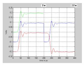
**Fig. 1** Various step signals for DFT/FFT processing. The example shown is a PSPL model 4022, 7.5 ps, TDR pulser measured by an HP 50 GHz oscilloscope.
