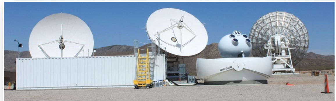
19-meter antennas in background LLGT gimbal on pedestal is ~4-meters tall
