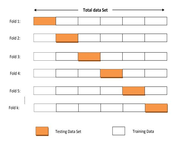
Figure 3: Process of k-fold cross validation
