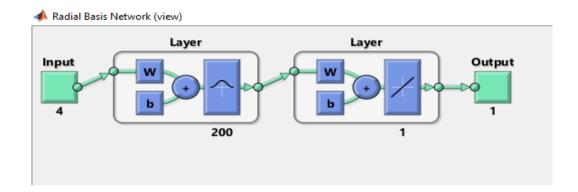
Figure 5: MATLAB generated view of RBFN through newrb() function of MATLAB.
