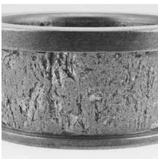
High loads and low speeds caused insufficient lubricant film on this tapered roller bearing inner ring.
