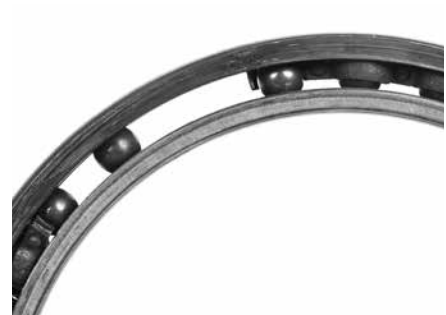
Cage damage from bearing lockup.
