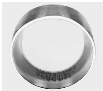
Deflection, inaccurate machining or wear of bearing seats caused an irregular roller path on this tapered roller bearing outer ring.
