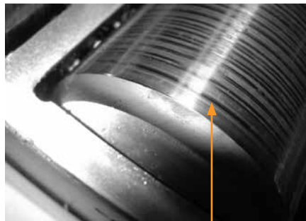
Circumferential grooving on rollers.
