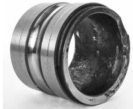
Fractured wide inner ring with locking collar due to undersized shaft
