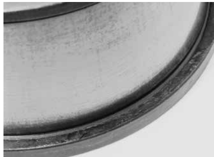
Rib and roller end heat damage.
