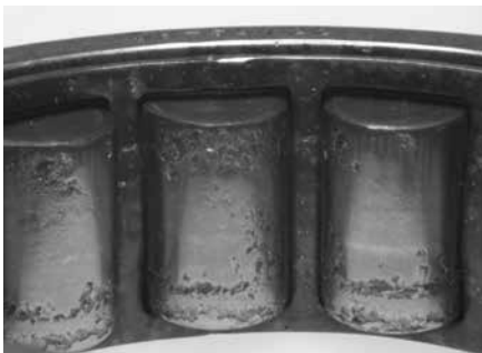
High loads resulted in fatigue spalling on this cylindrical roller bearing.
