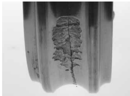
This ball bearing inner ring depicts fatigue spalling from high loads. The fracture is a secondary damage mode.
