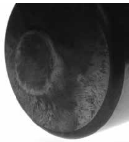
Roller end with adhesive wear.
