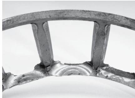
Cage pocket damage results from excessive roller movement.
