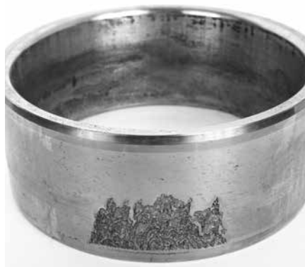
Heavy loads causing shaft deflection can lead to GSC spalling in this cylindrical roller bearing inner ring.
