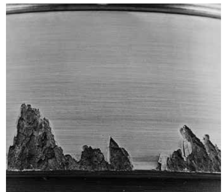
Geometric Stress Concentration (GSC) spalling.
