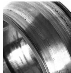
Adhesive wear on bearing inner ring.
