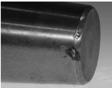
Roller with electric arc burns.
