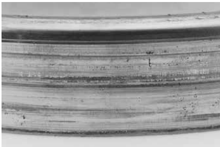
A loose outer ring fit in a rotating wheel hub (typically tight) caused this bearing race damage.
