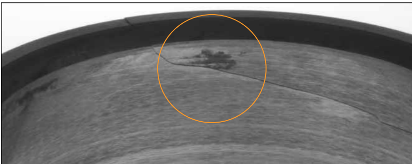
Fig. 52. This ball bearing inner ring fracture results from installation on top of a metal contaminant or raised metal nick.
