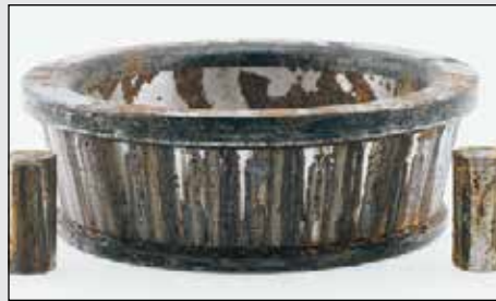
Fig. 75. A tapered roller bearing cone and rollers, and a ball bearing outer race and balls (Fig. 76) show rusting with pitting and corrosion from moisture/water exposure.
