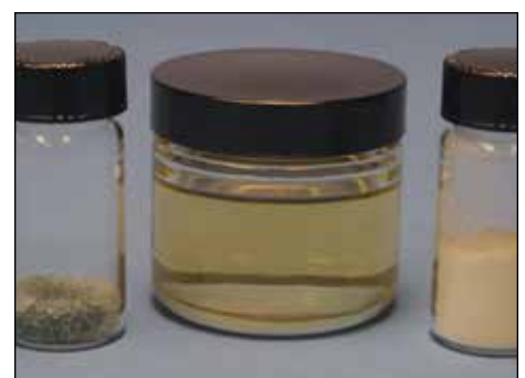
Fig. 71. Grease is a precise combination of additives, oil and thickener.
