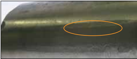
Fig. 68. This cylindrical roller flattened as a result of skidding
