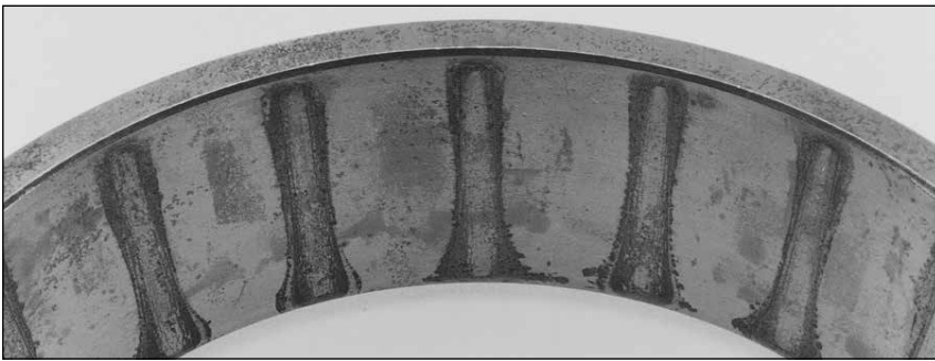
Fig. 12. This cup has heavy corrosion on the race. This type of corrosion may only be a surface stain without pitting. If the staining can be cleaned with a fine emery cloth or crocus cloth, the bearing may be reused. If there are pits that cannot be cleaned with light polishing, the bearing should either be discarded or, if practical, refurbished.
