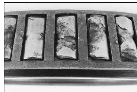
Fig. 30. A heavily overloaded tapered roller bearing resulted in premature, severe fatigue spalling on the rollers. The load was so heavy that large pieces of metal broke off the rollers.
