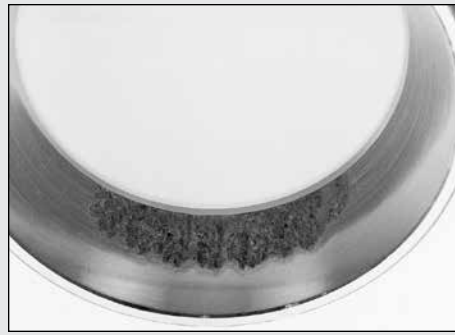
Fig. 37. This irregular roller path is 180 degrees opposite of Fig. 36.
