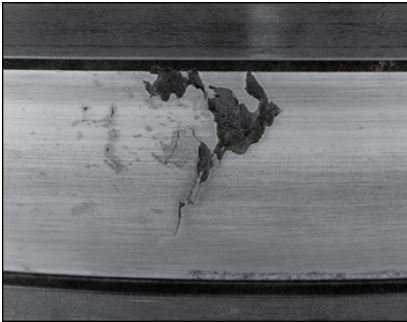
Fig. 5. A tapered roller bearing inner race (cone) with spalling from debris contamination bruises.
