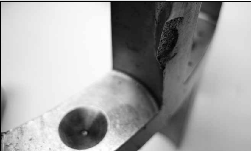
Fig. 45. Poor handling practices caused a deep dent on this spherical roller bearing cage bridge. This damage will result in a lack of proper roller rotation, possible roller skidding, increased temperatures and decreased life.
