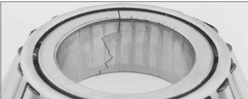
Fig. 53. An out-of-round or oversized shaft caused this fracture on a tapered roller bearing cone.
