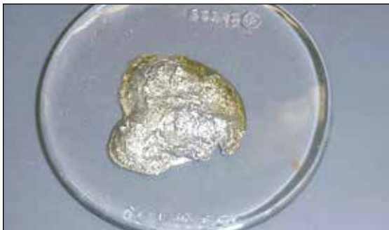
Fig. 67. Grease removed from an underfilled bearing shows shiny bearing metal debris.
