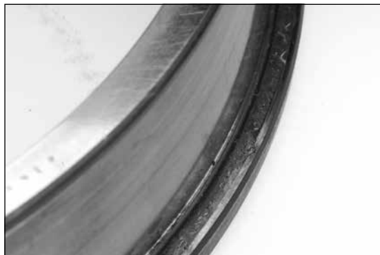
Fig. 19. Level 2 – Advanced rib scoring is due to inadequate lubricant film.
