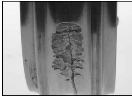
Fig. 27. This ball bearing inner ring depicts fatigue spalling from high loads. The fracture is a secondary damage mode.
