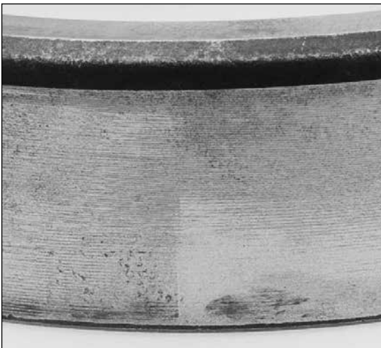
Fig. 48. The marks on the outside diameter of this cup race are caused by a high spot on the housing. The cup race is spalled at the spot that corresponds to the spot on the outside of the cup marked from heavy contact.
