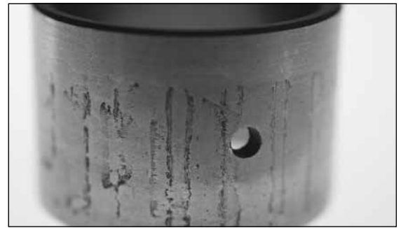
Fig. 13. This cylindrical bearing inner ring has etching and corrosion.
