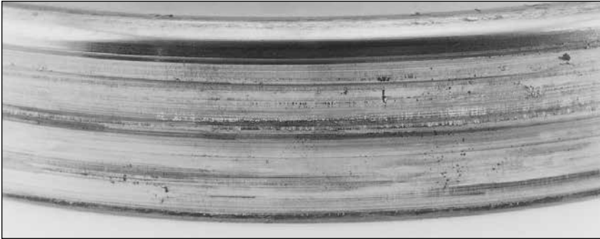
Fig. 50. A loose cup fit in a rotating wheel hub (typically tight) caused this bearing race damage.
