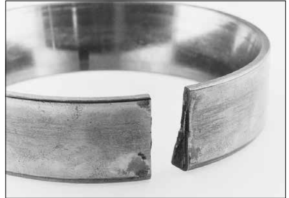
Fig. 51. This is what happens to a cup that is loose in a wheel hub. The cup turns and wears the cup seat so the fit becomes more loose. Then the cup starts to stretch or roll out. The cup, as it rolls out, continues to wear the cup seat and the cup continues to stretch. This process continues to the point where the stretch of the metal reaches the breaking point and the cup cracks open.
