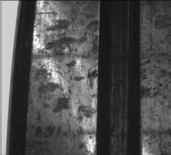
Fig. 46. A worn-out housing caused this bearing to lose fit and fret (move) during service. As a result, metal tearing and wear occurred on this spherical outer ring.
