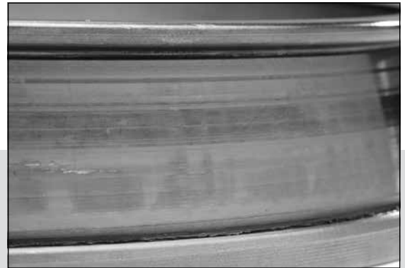
Fig. 17. Level 1 – Discoloration due to elevated operating temperatures.
