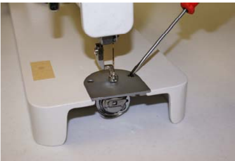
Remove the two needle plate screws from your machine.
