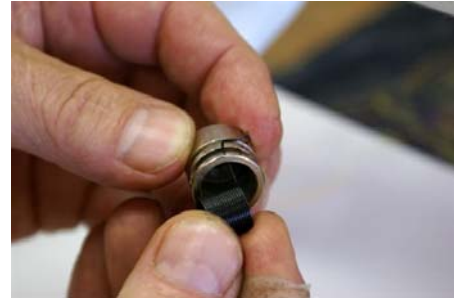
Fig 15: Twist while inserting new spring
