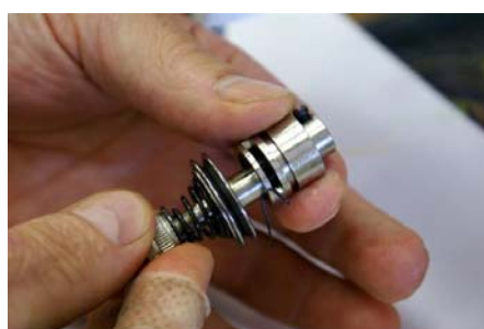
Fig 8: Remove tension assembly from barrel
