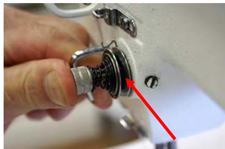
Fig 23: Press in and notice the tension disk opens
