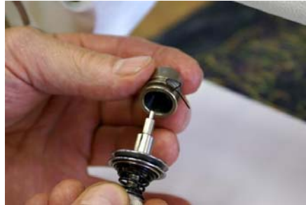
Fig 17: Insert the tension assembly back in barrel
