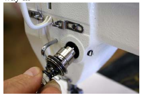
Fig 21: Place the assembly back into your machine
