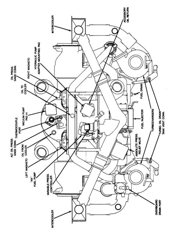
Figure 7-2. Installation Drawing – Rear View – TIO-540-AE2A
