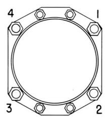
Figure 5-2. Sequence of Tightening Cylinder Base Hold-Down Nuts
