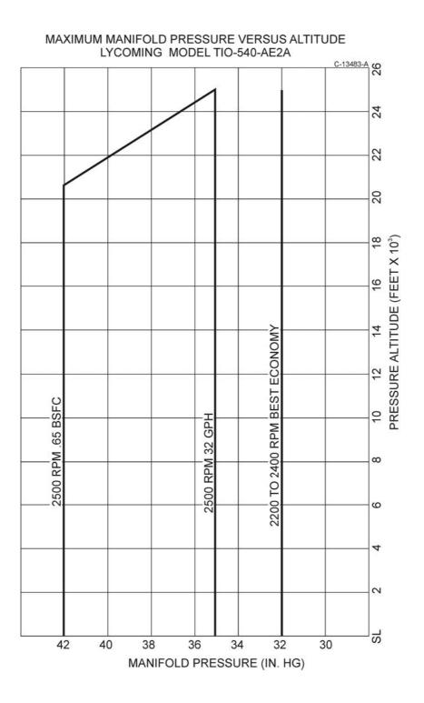
Figure 3-2. Maximum Manifold Pressure vs. Altitude
