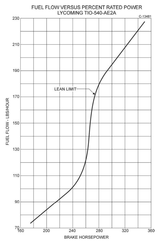
Figure 3-3. Fuel Flow vs Percent Rated Power
