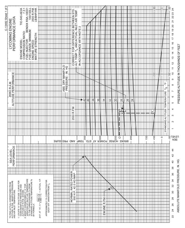
Figure 3-4. Sea Level/Altitude Performance Curve – (Sheet 1 of 3)
