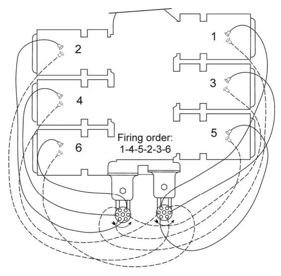
Figure 5-1. Ignition Wiring Diagram
