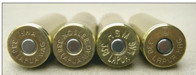
Above, assorted brass showed variances in how it handled .338 Lapua pressures. Right, NoslerCustom brass and Federal 215 Large Rifle Magnum primers were used for developing most of the load data.
