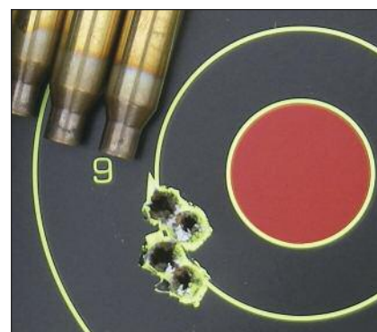
This four-shot group with Remington ammunition measures .782 inch and was fired at 200 yards from the Savage Model 110 BA test rifle.
