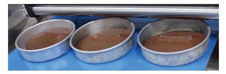
**FACTOR FOUR** — **SPECIFIC GRAVITY.** The Specific gravity is an important factor when depositing aerated batters. Typically, the recharge speed needs to be reduced if tunneling in the hopper happens. This would be the case of a very light batter in which the high recharge speed makes the air enter through hidden passages created in the depositor hopper. When the batter is very aerated, its delicate micro-air-bubble structure may easily break.
