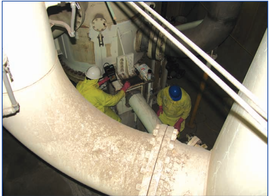
Fig. 1 — Ultrasonic examination being performed on heat exchanger supports. Even if you’ve performed similar inspections in the past, you need to properly and thoroughly prepare for each inspection job.
