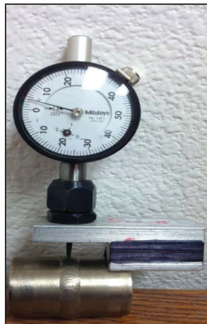
Fig. 2 — Typical dial indicator used to check mismatch, convexity, concavity, and other conditions.
