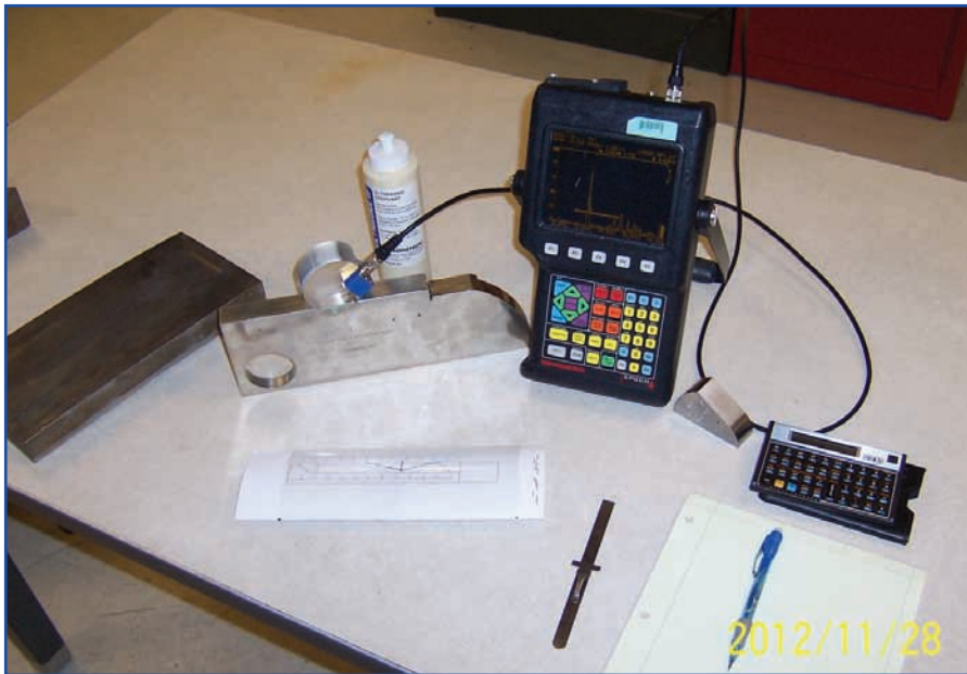
Fig. 2 — Typical ultrasonic examination equipment for applications to the requirements of AWS D1.1, Structural Welding Code — Steel. Don't rely solely on your memory, check the code requirements.
