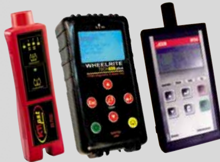
A small sampling of existing major TPMS scan tools that are compatible with the REDI-Sensor Universal Transmitter.
