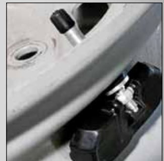
Valve options for 0.453", 0.625", and 7.7mm rim holes
