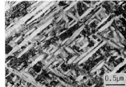
Fig. 13: Bright field micrograph of \alpha platelets in the Ti-alloy \beta -CEZ aged for 8h at 580°C (TEM).
