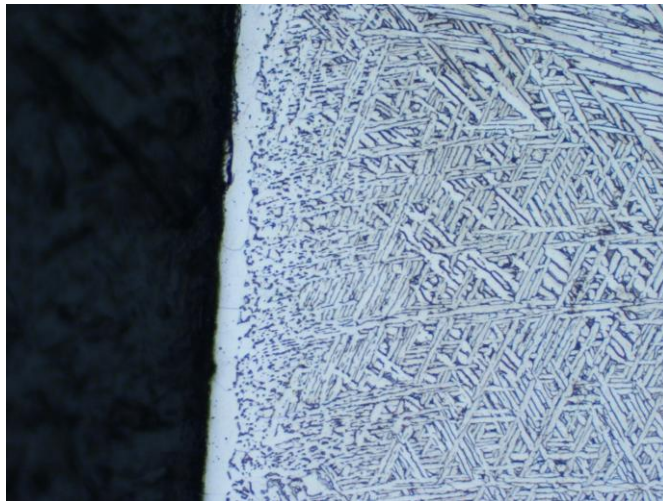
Figure 17: Uncoated Ti-6-4 vacuum heated sample
