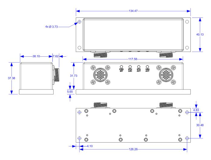
Figure 2. eNet-MA4 Dimensions (mm)
