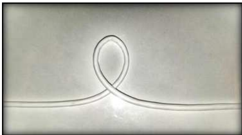
Figure-04: Bending the cable more than maximum Allowed bending radius
