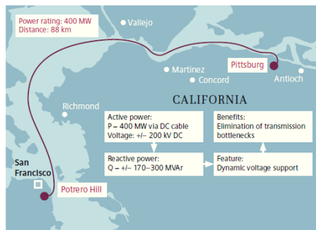
Fig. 8 MMC-based HVDC Trans Bay Project [19].
