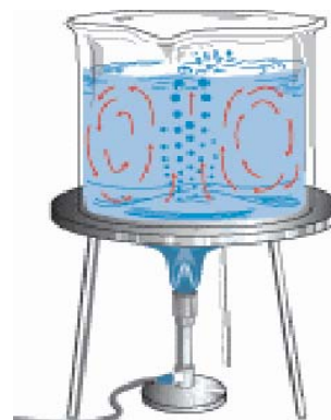
Figure 4: Convection currents in boiling water
