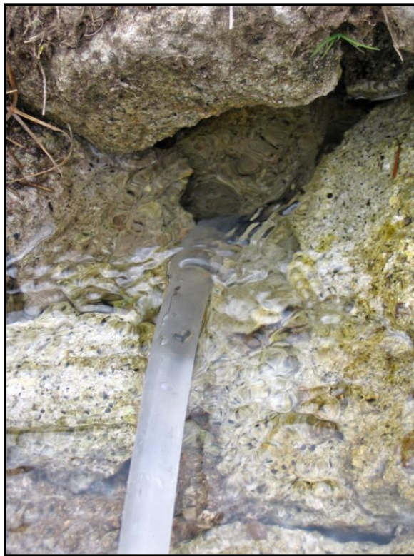
Figure 5.8: Plumbing methodology used to sample springflow from within the fractured bedrock.
