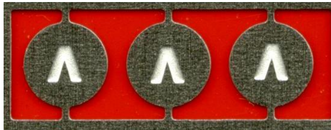
Figure 6 – Color imaging for inspecting partial etch features
