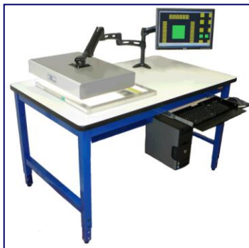
Figure 1 – Low-cost, flexible inspection system
